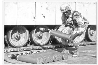
An ammunition specialist carries a 105mm armorpiercing, discarding sabot round, to be used in an M-1 Abrams main battle tank, during Operation Desert Shield. Photo by Army Sgt. Brian Cumper
