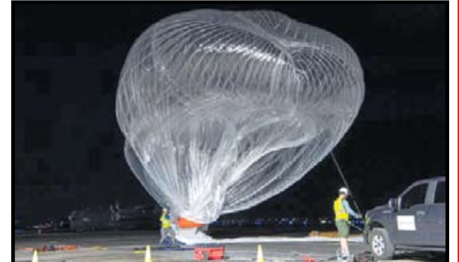
Valiant Shield Flight ops personnel prepare to launch a high-altitude balloon in support of Exercise Valiant Shield 2024 at Antonio B. Won Pat International Airport, Guam, June 10, 2024. The balloons provide the military with long endurance and persistent air-based capabilities that serve as a platform for different payloads such as sensors, communication relays, and weather monitoring systems. U.S. Air Force photo
