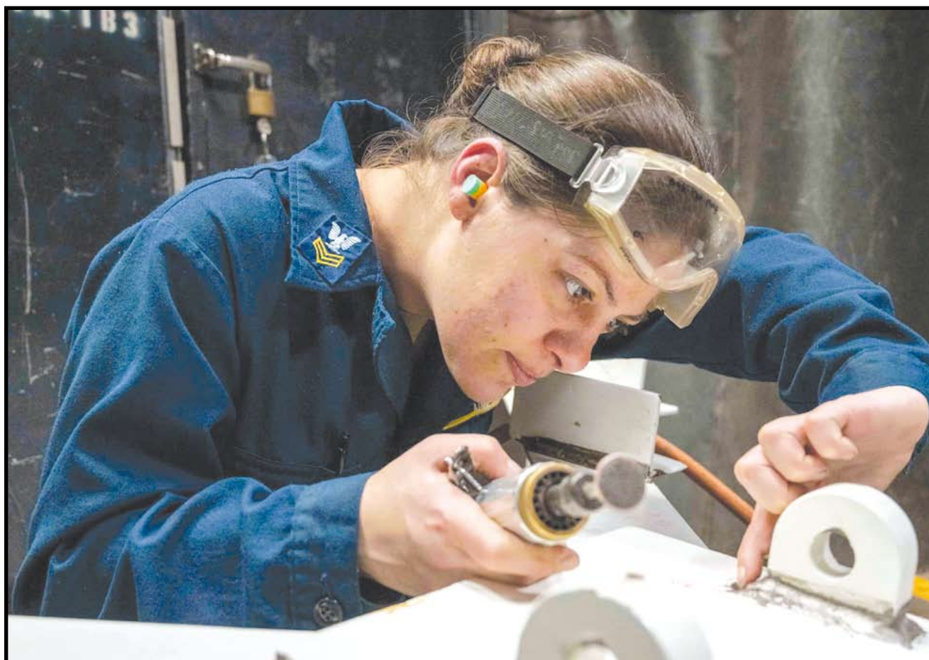
WELDING FOCUS Navy Petty Officer 1st Class Tigar Oneil prepares to fix a crack in an x-beam aboard USS Nimitz in the Pacific Ocean, late last year. U.S. Navy photo by Petty Officer 2nd Class Caylen McCutcheon
