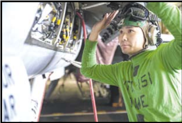
ANOTHER DAY AT THE OFFICE Aviation Structural Mechanic (Equipment) Zhibin He conducts testing on an oxygen generation system of a Super Hornet aboard Abraham Lincoln aircraft carrier underway July 28, 2025. U.S. Navy photo by MC3 Jordan Steis
